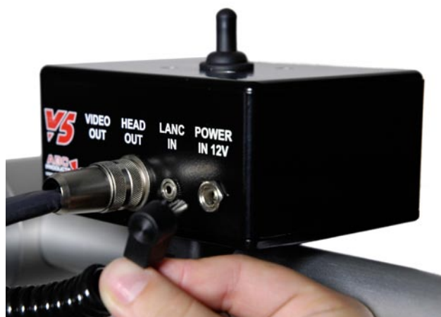
2. Attaching control cables at the control unit.
